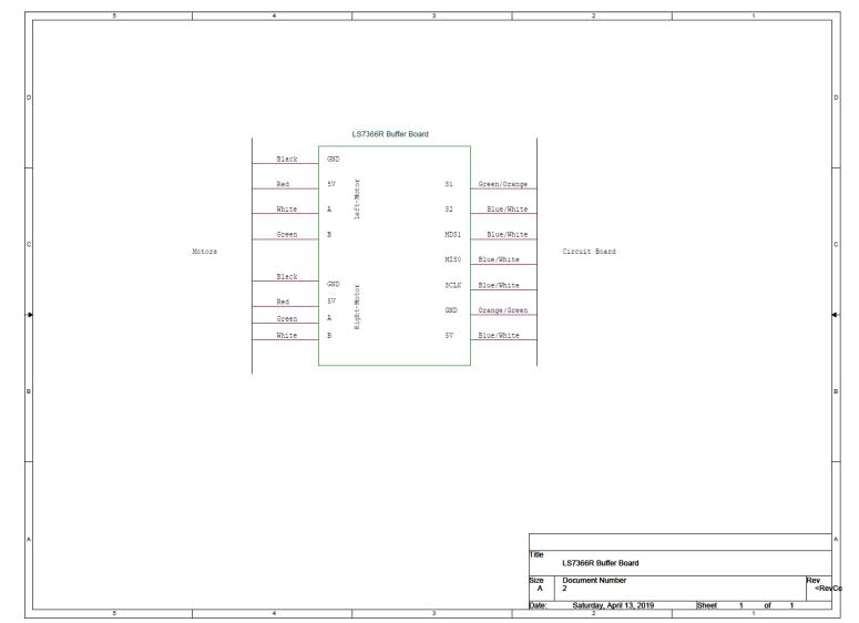
B-3. Schematic representation of the LS7366R Buffer Board wired to two motors with color coordinated wires going into the circuit board.
