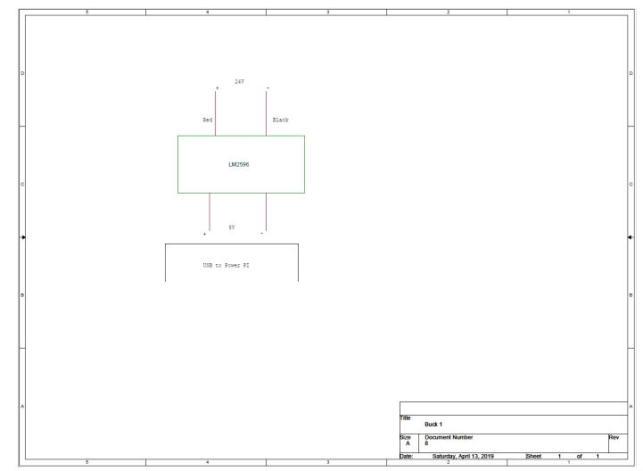
B-1. Wiring diagram schematic of a DC-DC buck converter stepping down 24 volts to 5 volts to power the Raspberry Pi.
