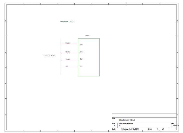
B-10. Four ultrasonic sensors are used all around, there wiring is identical among all four. A representation of their wiring is illustrated in the schematic.
